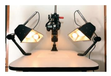
Fig. 1. The digital image analysis system showing specimen position, standardised lighting and camera position.
